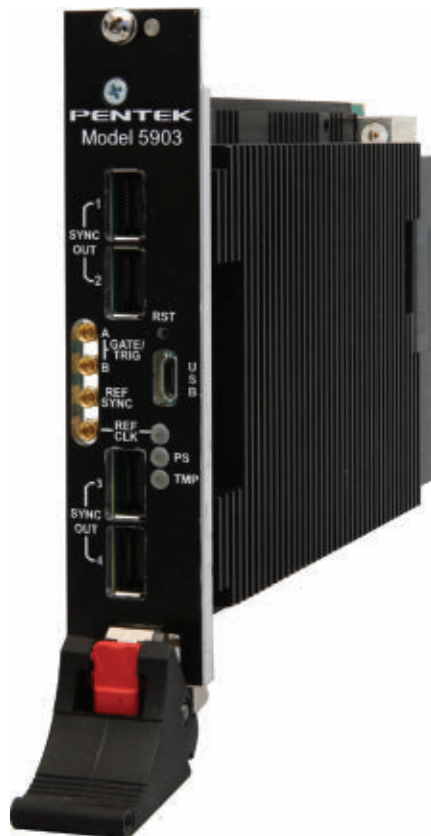
The Pentek model 5903 can synchronize as many as eight RF systems-on-chip (RFSoc) products to support 64 elements of a 5G phased-array communications antenna.
