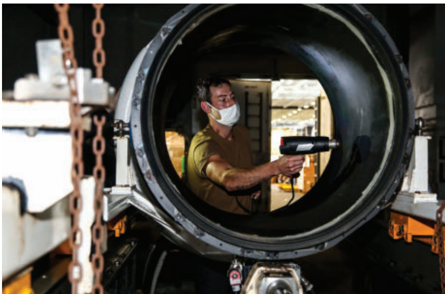
An aviation machinist's mate aboard the aircraft carrier USS Abraham Lincoln performs a liquid crystal test to reveal possible delamination of an engine run trailer.
